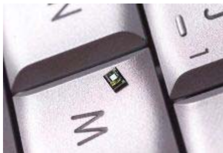
AKU2000 Digital MEMS Microphone - bare die on PC keyboard
